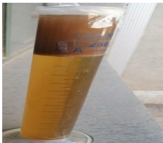
Figure 1: two phases of the solution; the upper phase, which contains ethyl acetate and Alternaria secondary metabolites and lower phase consisting of water.
